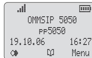
The name of the communications system is “OMMSIP” and the handset has the internal phone number “5050”. The handset receives this information from the communications system. The name of the handset is “pp5050”. You can edit this name in the “Telephone Options > User Name” menu.
