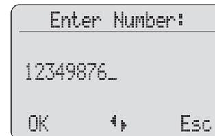
Enter "12349876\_", for example. You can correct your input by using the arrow keys to move the cursor to a digit, which will then flash. Press the C-key to delete the digit to the left of the flashing character. You can then insert new digits at this point. When you have completed your input, press **OK** to move to name input.
