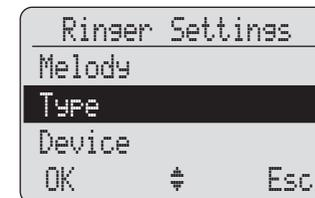
Use the arrow keys to select one of the submenu items Melody, Type, Device and Volume Settings, e.g., **Type**, and press **OK**.
